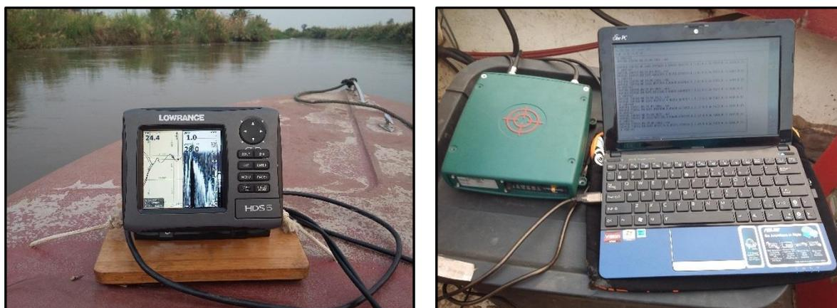
**Figure 5.3** Bathymetric survey of the Shire River and Namichimba distributaries. Left: Lowrance HDS5 sonar equipment; right: Veripos LD7 DGPS connected to laptop for logging of the NMEA output string
