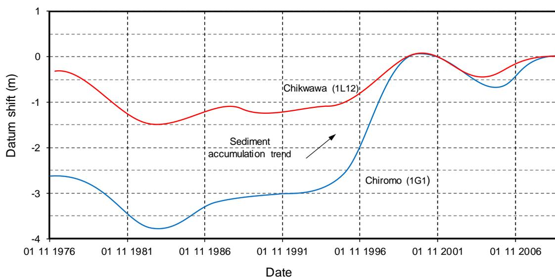
**Figure 6.18 Datum-shifts (smoothened) at the Chikwawa and Chiromo hydrometric stations over the period 1976 to 2009, derived from differences between observed water levels and modelled stages using the existing physical template,<sup>357</sup> an increase in datum over time infers sediment accumulation**
