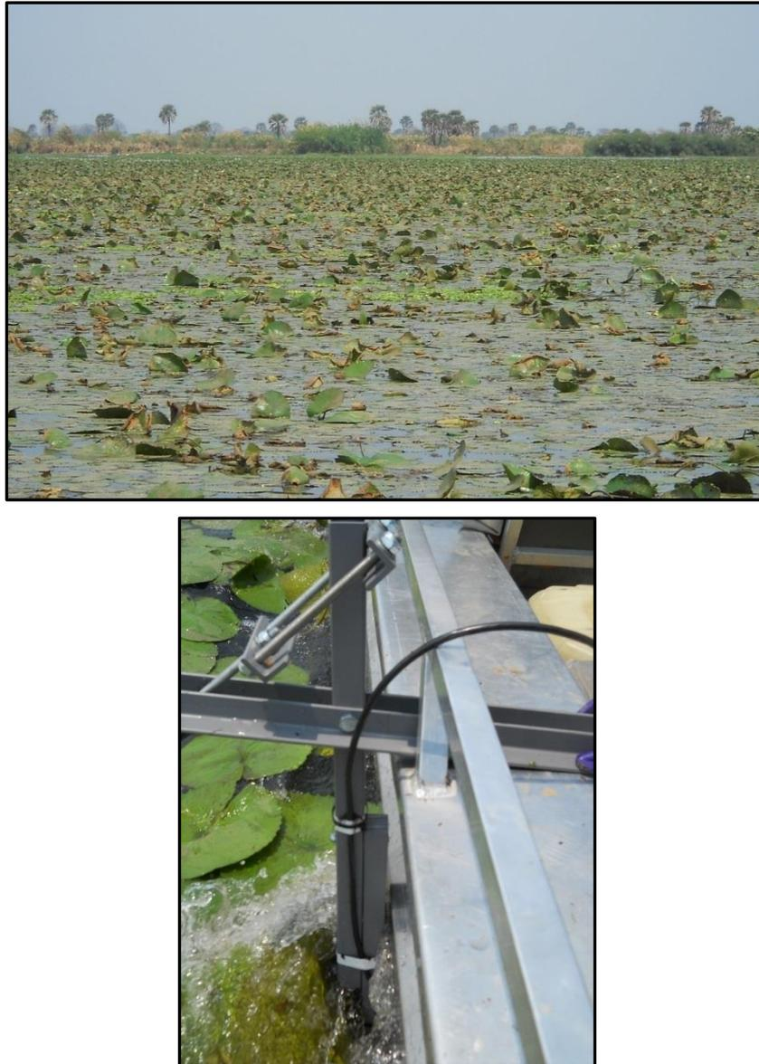
**Figure 5.2** Top: extensive coverage on the surface of a shallow lake by floating-leaved aquatic plants, making sonar surveys difficult; bottom: purpose-designed attachment fixed to the side of the airboat which was effective in parting dense mats of floating-leaved aquatic vegetation, allowing sonar pulses to penetrate the water depth
