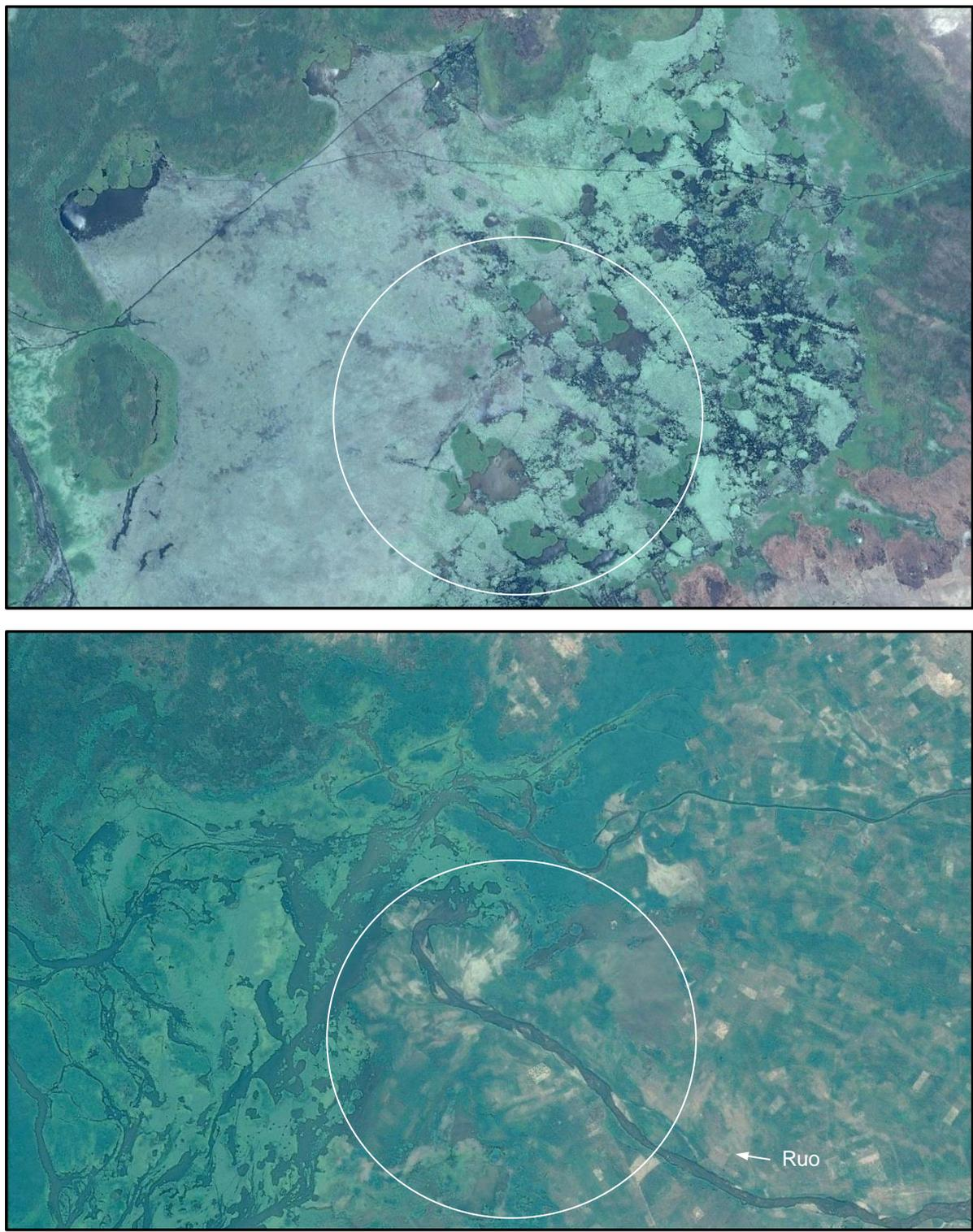
**Figure 4.25** High resolution satellite imagery (Google Earth) showing substantial diminution of the north-eastern extent of Lake Tomaninjobi due to sediment deposited by the Ruo River, following its re-routing through the Marsh in January; top: 27 December 2013; bottom: 27 September 2016; floating-leaved aquatic vegetation displays as white/pale-green; the spatial extent of the areas in this figure is indicated in Figure 4.24
